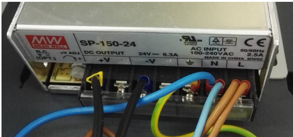
Drawing 7. Mamos power supply; Heated filter might be connected to 3 pins on the right: ⊕ - Earth, N – Neutral, L – Line
